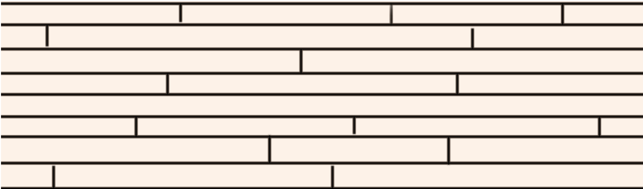
(pic1) Staggering board randomly adds strength to the total floor
